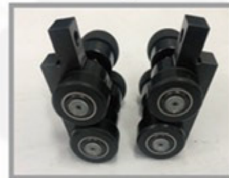
輔助挾持滾輪組 Auxiliary clamping roller set
