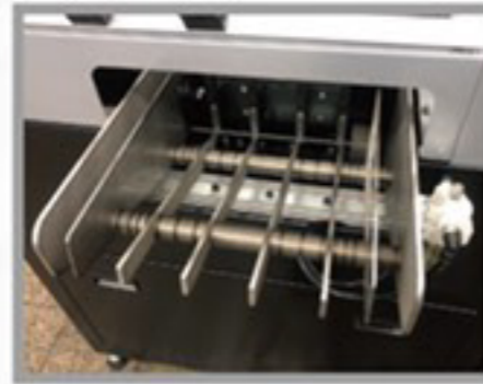
長度可調式入料槽 Length adjustable feed tank
